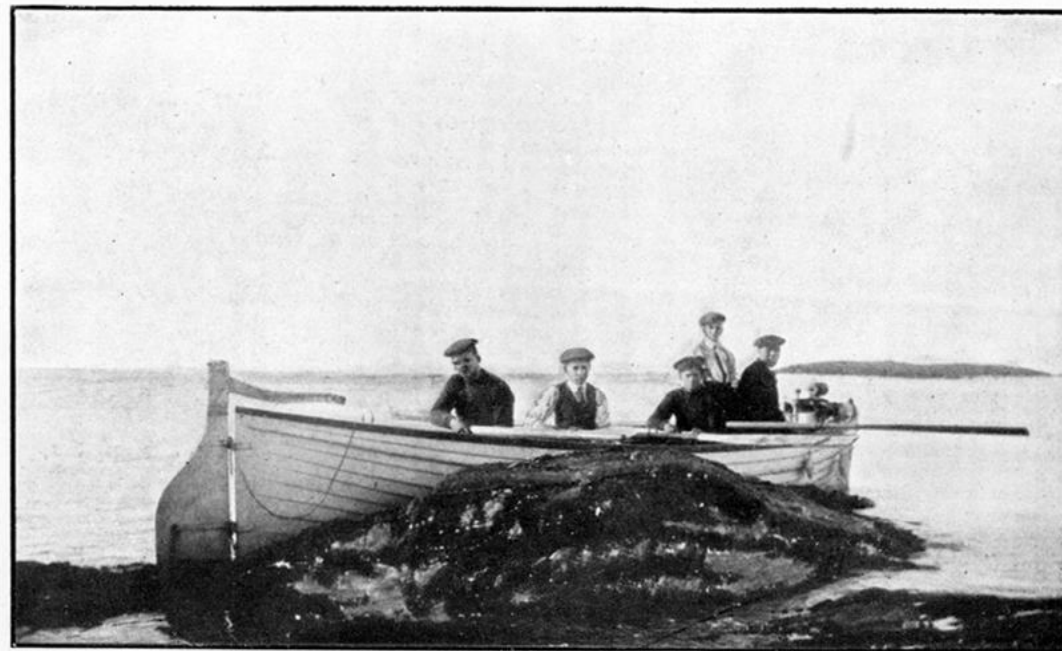
(ii.) Acoustic survey carried out from a ship's boat. The phonometer is shown mounted at the bow of the boat. The results obtained are shown graphically in Chart 2.
